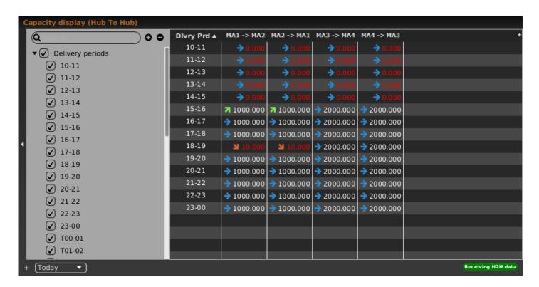
The configured threshold value is applied to the entire capacity matrix, i.e. to all paths in the capacity matrix. For the threshold configuration see *General*.
