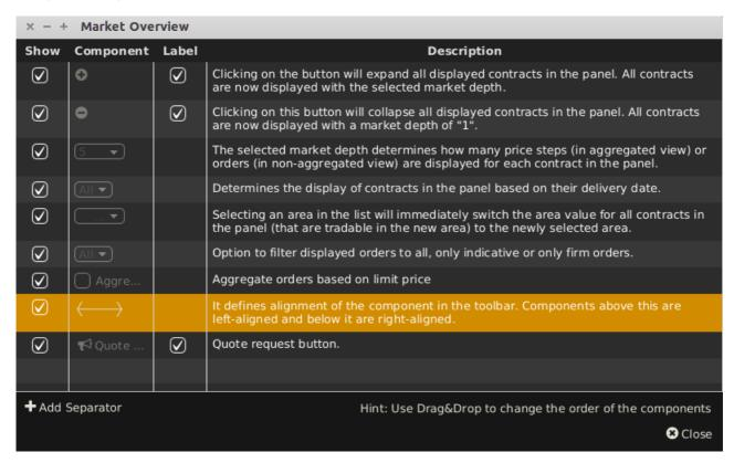
In the "Component" column it is possible to see how each item will appear in the bottom bar: as a toggle button with a text placeholder, a box with its label or an icon. The label can be hidden by unchecking the box in the "Label" column. The last column contains the description of the item.
