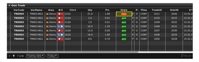
If a recall request has been rejected, the trade status is changed to "RECALL REJECTED":
