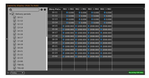
A Delivery Period can be added to or removed from the main table of the panel (also called capacity matrix) by ticking or unticking the respective box in the navigator. After being ticked a new row with the Delivery Period will be added to the capacity matrix with the latest ATC values for the selected paths (see *Adding and Removing Paths between Areas*)
